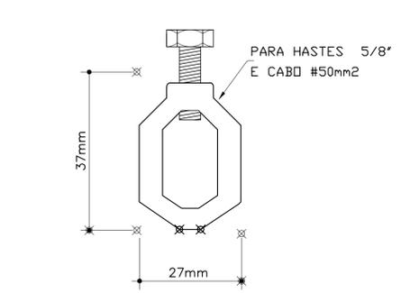
CONECTOR CABO/HASTE EM BRONZE DETALHE GENÉRICO SEM ESCALA
